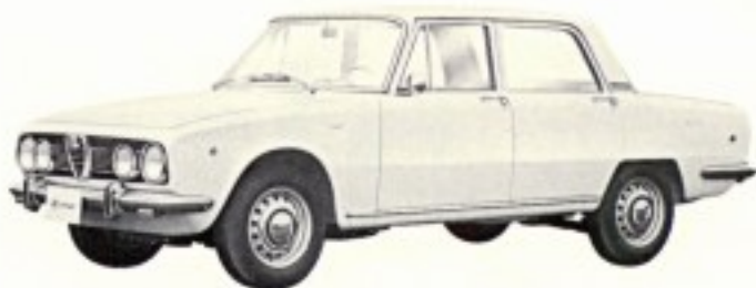
1750 Berlina Five-passenger 4-door sports sedan. Four cylinders, 1779 cc. 132 hp (SAE). Over 112 mph.
