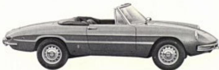
1750 Spider Veloce ® Two-seater sports car. Four cylinders, 1779 cc. 132 hp (SAE). Over 118 mph.
