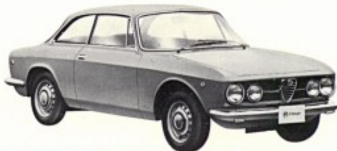
1750 GT Veloce ® Luxury sports coupe with two bucket seats, 2 occasional seats. Four cylinders, 1779 cc. 132 hp (SAE). Over 118 mph.
